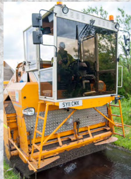
The spreader width is constantly adjusted to fit the road width precisely
